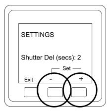
To set the shutter delay press the "-" and "+" buttons
