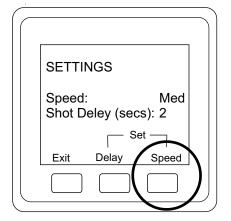
To change the turntable speed press the "Speed" button.
