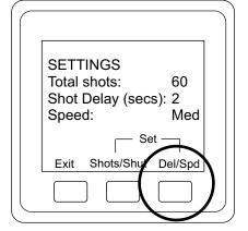
To set the delay before taking a shot or the speed of the turntable press the "Del/Spd" button.
