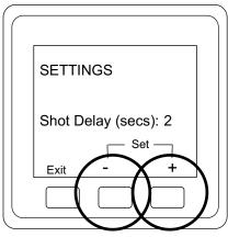
To set the shutter delay press the "-" and "+" buttons.
