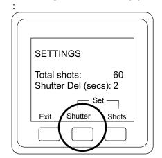
To change the shutter delay press the "Shutter" button
