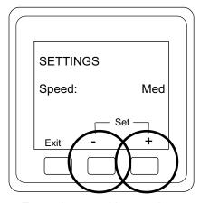
To set the turntable speed press the "-" and "+" buttons.
